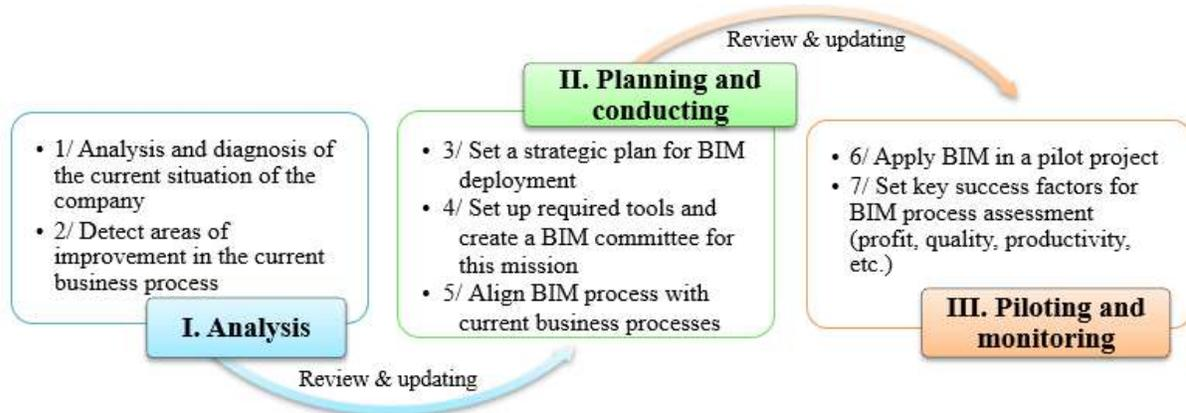
**Figure 20: The main steps of BIM deployment.**
